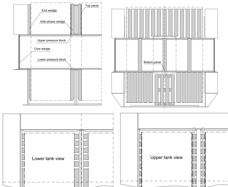
Figure 12 – Structural parts of a shell type transformer
