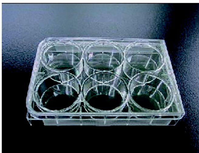
Figure 2 — 6 wells plastic plate for plaque assay
