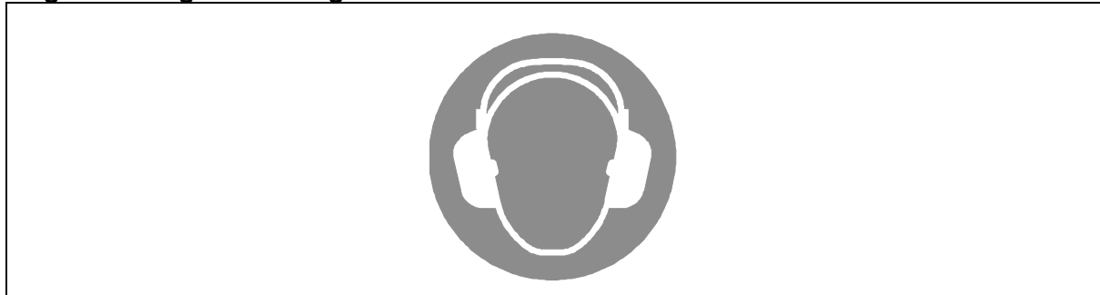
Figure 7 – Sign indicating areas where visual alarm devices are needed
