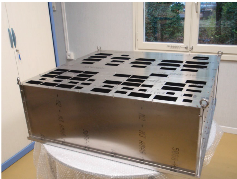
Figure A.3 — plate, collimator and front mask before painting
