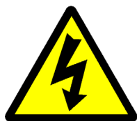
Figure 208 - Hazardous voltage logo according to ISO 7010 – W012
