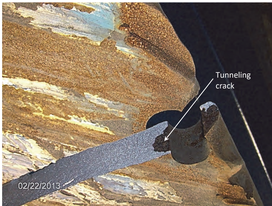
Figure 3-2. Crack Tip Tunneling Contributing to a Missed Crack Tip That Later Fractured
