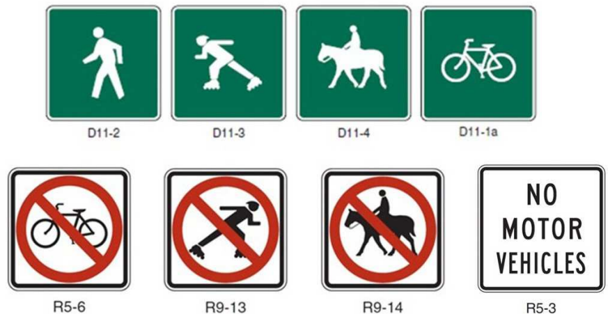
Figure 2-14. Mode-Specific Guide and Selective Exclusion Signs (FHWA, 2009)
