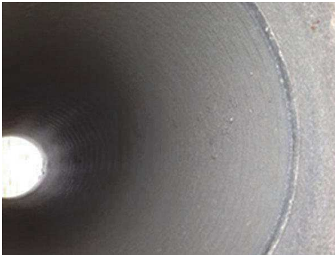
Figure 8 —Acceptable Rifling ( Photo Courtesy of ACPA )
