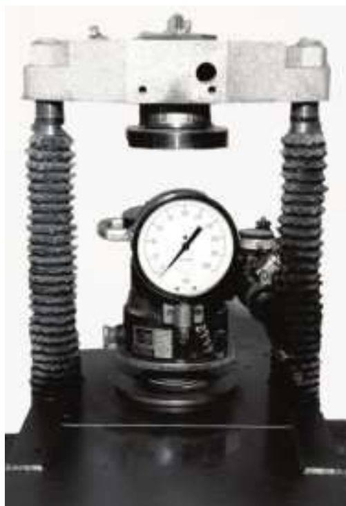
Figure 3 —Hveem Stabilometer Mounted in the Testing Machine
