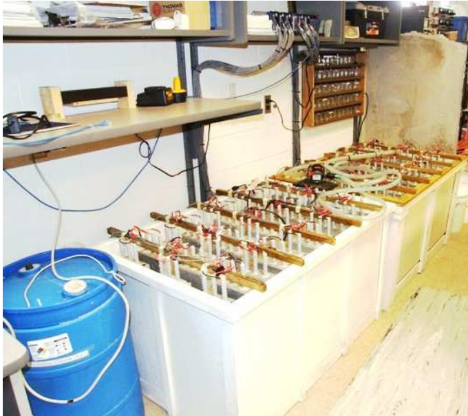
Figure 1 —Tombstone Test Set-Up. (The 3 percent saltwater storage tank is located in the lower left corner, with the tombstone immersion tanks adjacent to the saltwater storage tank, and the data acquisition system above the tombstone tanks at the top of the photo).
