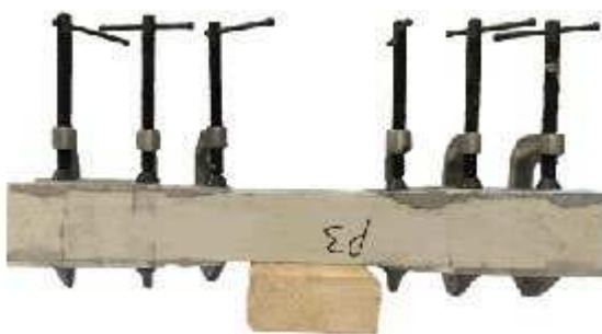
(e) Clamping of One Test Specimen with Six C-Clamps
