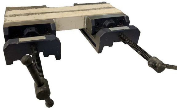
(f) Clamping of Two Test Specimens with Two Vise Clamps
