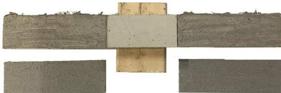
(c) Adhesive Application on Test Specimen and Transfer Plates
