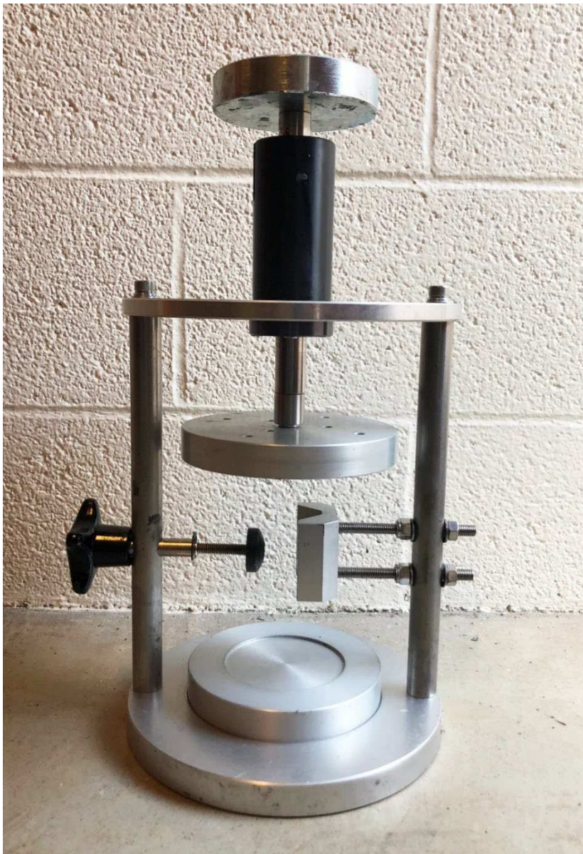
Figure 5 —Example of a Loading Platen Gluing Apparatus
