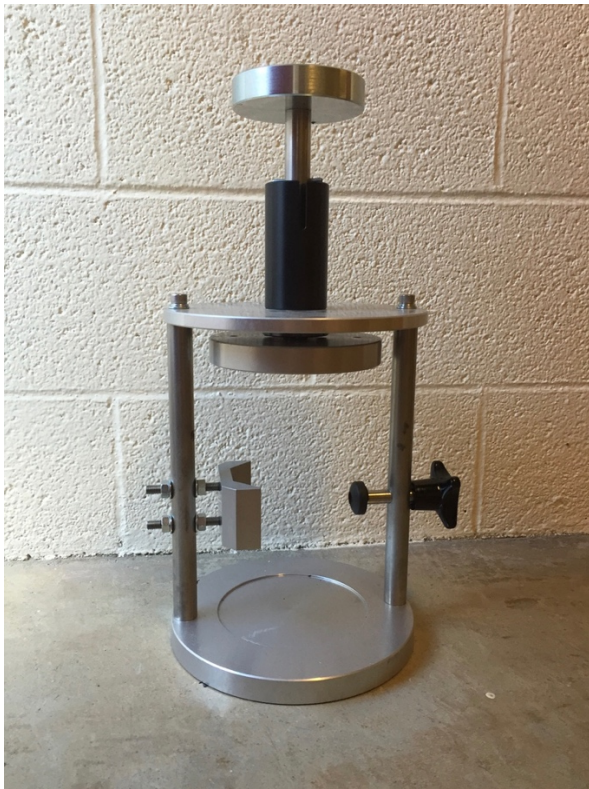
Figure 3 —End Plate Gluing Apparatus
