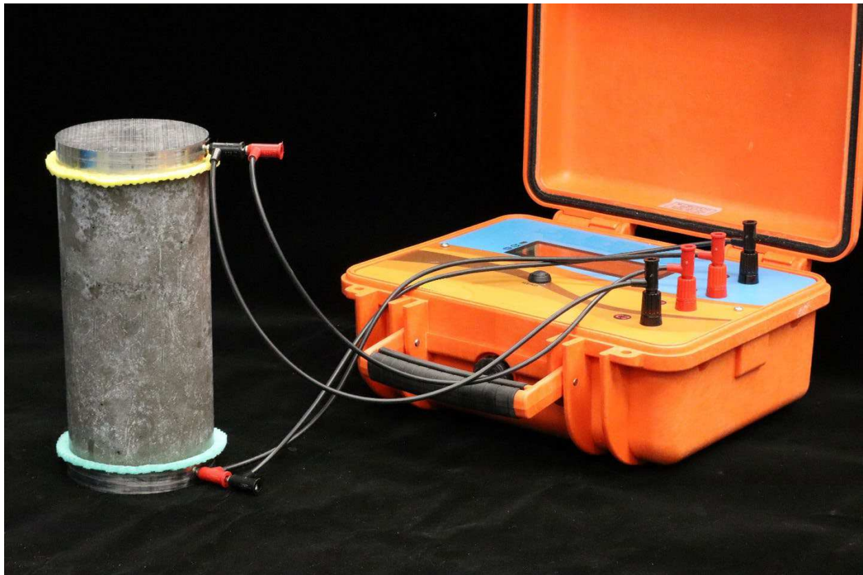
Figure 1 —Test Setup for Determination of Uniaxial Resistivity
