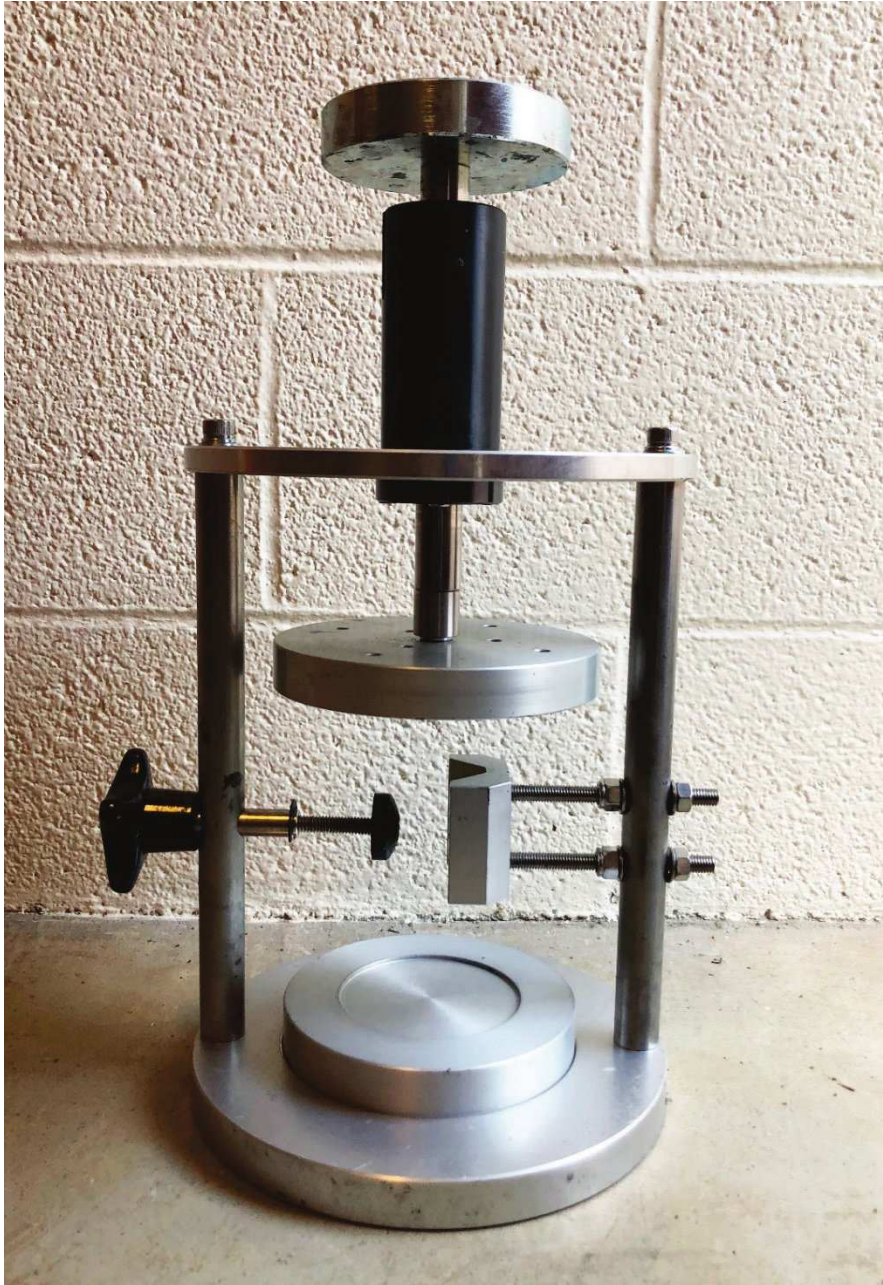
Figure 5 —Example of a Loading Platen Gluing Apparatus
