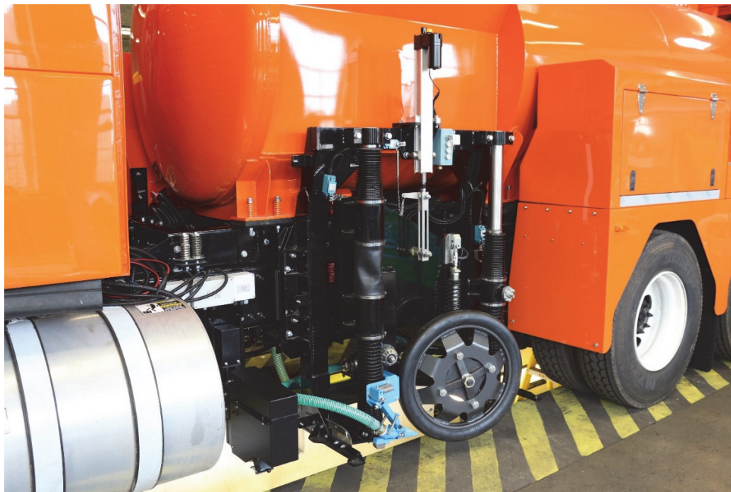
Figure 1 —Device Wheel Assembly for a Machine with the Wheel in Its Raised Position
