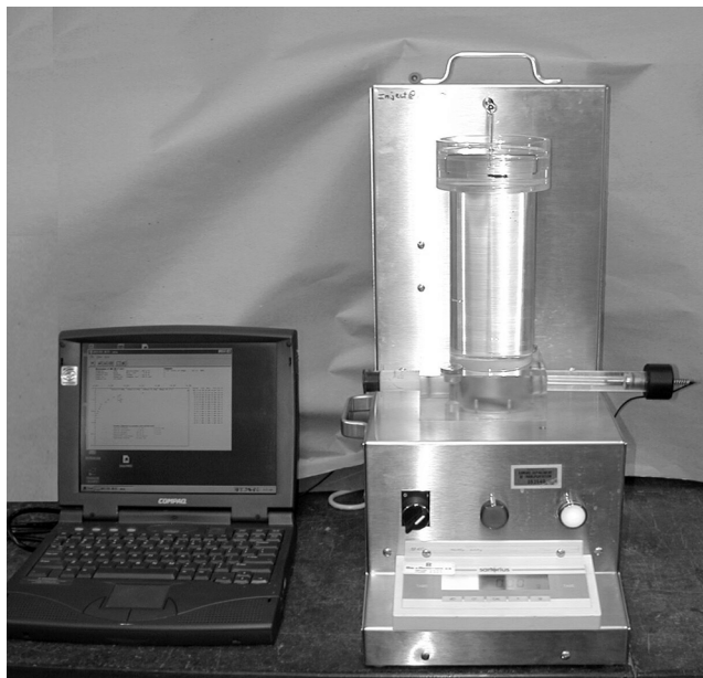
Figure 2 —Typical Apparatus with Riser Cylinder, Cabinet, and Computer
