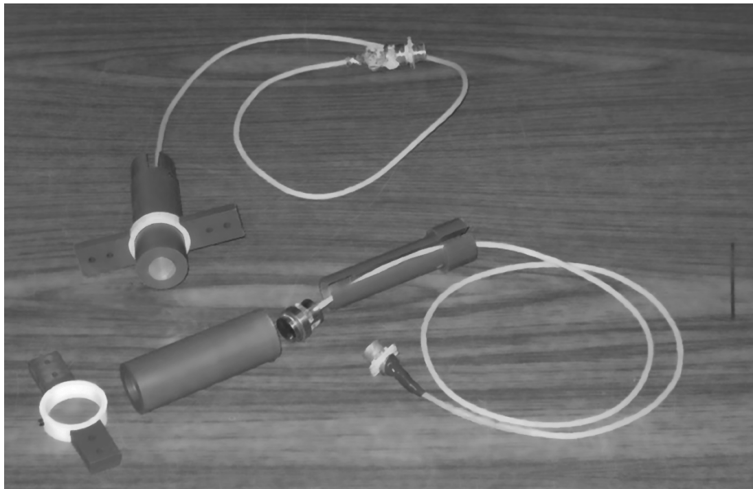
Figure 2 —Bracket for Attaching Pressure Transducer to Formwork
