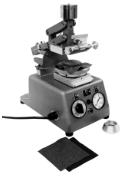
Fig. 2—C.S.I. Surface Abrader prepared for frosting test.
