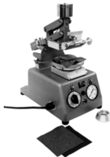
Fig. 1—Universal Wear Tester prepared for frosting test.
