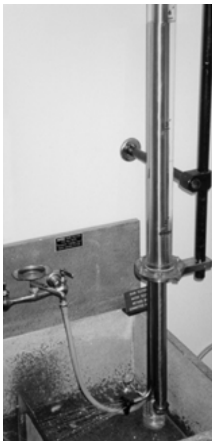
Fig. 1—Rain tester, complete assembly.
