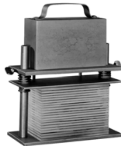
Fig. 1—Horizontal perspiration tester.
