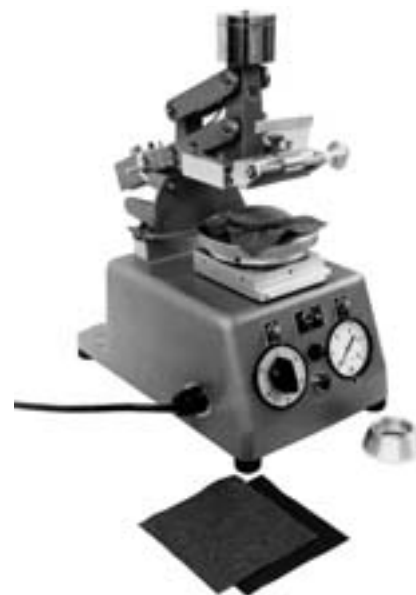
Fig. 1—Universal Wear Tester prepared for frosting test.
