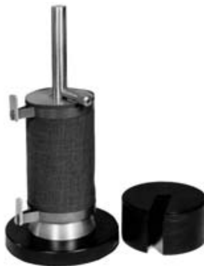
Fig. 1—AATCC Wrinkle Tester.
