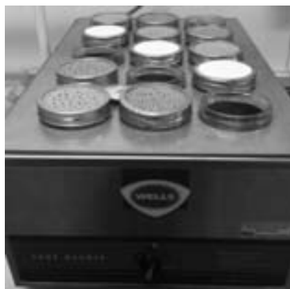
Fig. 2—Test apparatus with 8 test specimens, 3 control specimens, and 4 empty jars (see 11.3.1).
