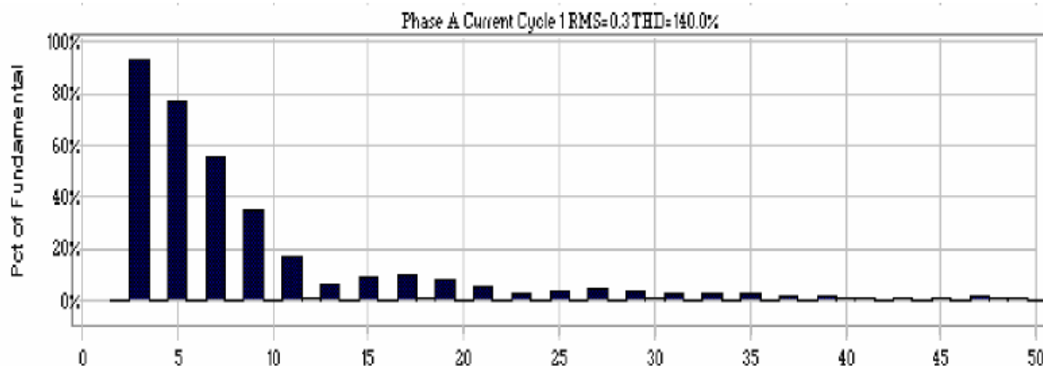
FIGURE 7 Harmonic Spectrum of Currents Drawn by Computer Switched Mode Power Supply
