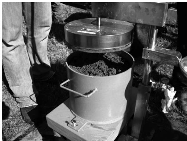
Fig. 3.1—ASTM C1170 Vebe consistency test apparatus with 27.5 lb (12 kg) surcharge. (Photo courtesy of U.S. Department of Agriculture, National Resources Conservation Service, 2008.)
