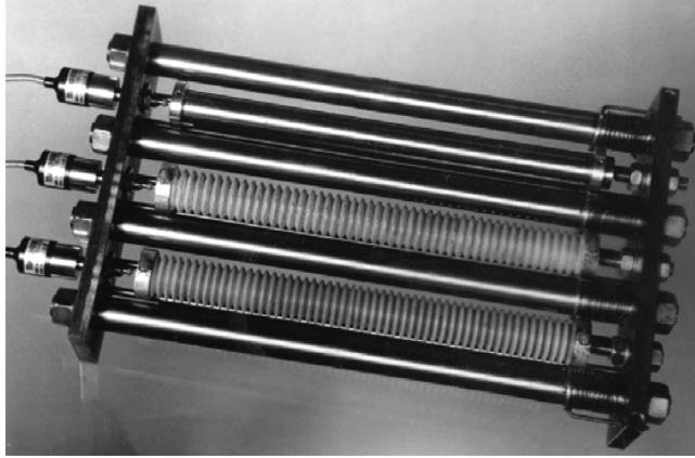
Fig. 4.5—Dilatometer with corrugated modulus for measurement of linear autogenous shrinkage of cement paste (Jensen and Hansen 1995).
