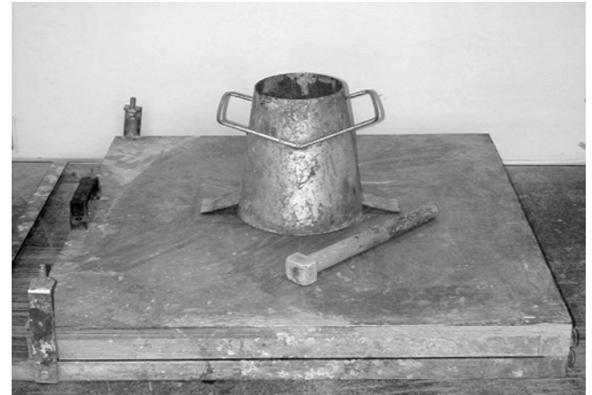
Fig. 3.12—Flow table test apparatus (1 mm = 0.039 in.).
