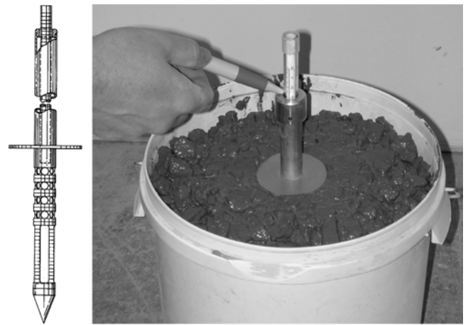
Fig. 3.3— K -slump tester (U.S. Patent and Trademark Office 1975).
