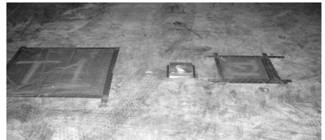
Fig. 3.2—Even though plastic sheet tests can show no evidence of moisture, calcium chloride tests conducted on adjacent concrete can indicate moisture vapor emission rates as high as 13 lb/1000 ft 2 /24 h (6.3 kg/100 m 2 /24 h) (Suprenant 2003b; Kanare 2005).
