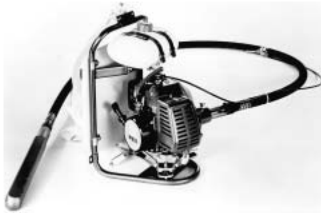
Fig. 5.1(b)—Backpack two-cycle gasoline engine-driven vibrator.
