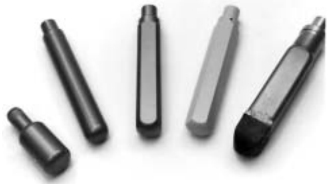
Fig. 5.4—Several of the different sizes and shapes of vibrator heads available. From left to right: short head, round head, square head, hexagonal head, and rubber-tipped head.
