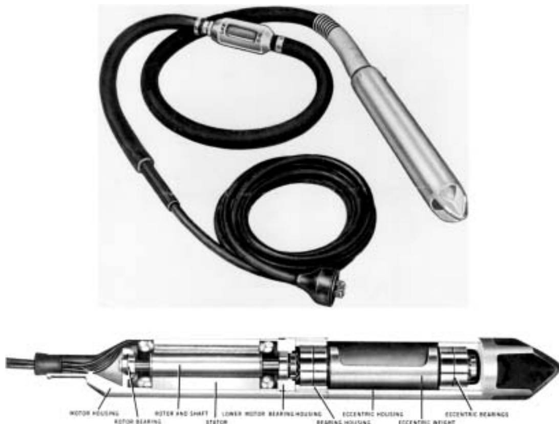
Fig. 5.2—Electric motor-in-head vibrator; external appearance (top) and internal construction of head (bottom).
