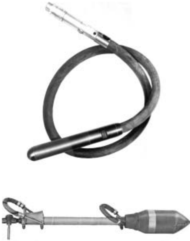
Fig. 5.3—Air vibrators for ordinary construction (top) and for mass concrete (bottom).
