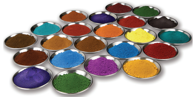
Fig. 4.2—Pigments added to concrete mixtures as dry powders or as liquid solutions offer a wide range of color options (courtesy of Davis Colors).
