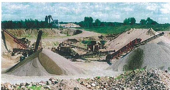
Fig. 3.3—Aggregate stockpiles are difficult to sample properly.
