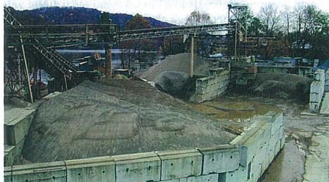
Fig. 4.2—Keep aggregate piles clean and separate to minimize segregation.
