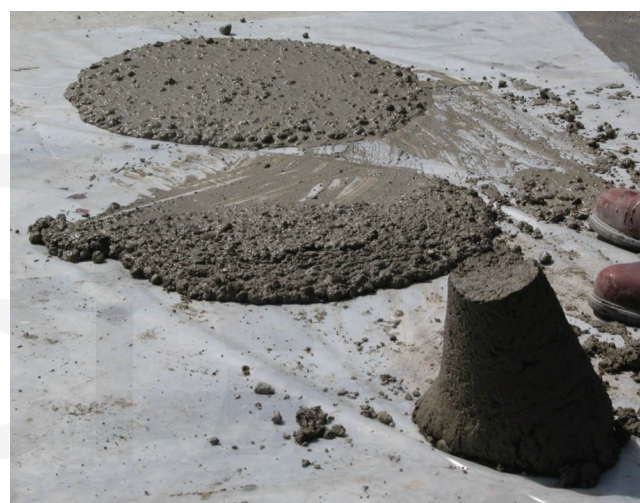
Fig. 3.3.1.2—Modified slump test for measuring flowability of SCC.
