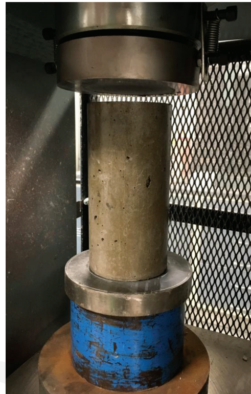
Fig. 3.3.2.1—A concrete cylinder in a test rig is loaded vertically until failure. (Photo courtesy of Portland Cement Association.)
