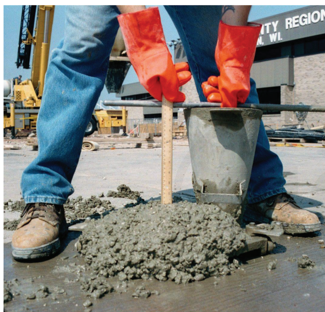
Fig. 3.3.1.1b—Slump test for consistency of concrete illustrating a high slump.
