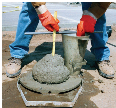
Fig. 3.3.1.1c—Slump test for consistency of concrete illustrating a low slump.
