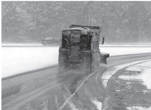
Fig. 4.1g—Application of deicing chemicals to roadways.
