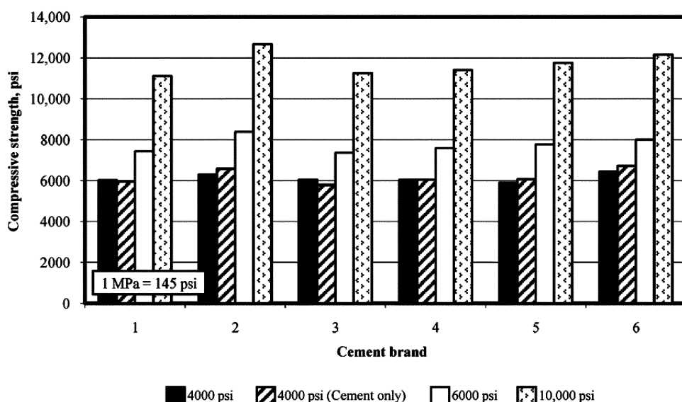
Fig. 4.4—Effects of various brands of cement on concrete compressive strength using different mixture proportions. (Mixture proportions shown in Tables 4.1(a) and (b).)
