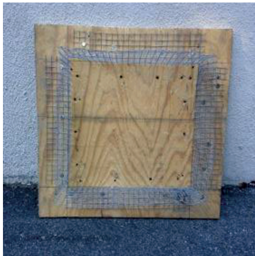
Fig. 1.6.3.1a—Material test panel with hardware cloth sides.
