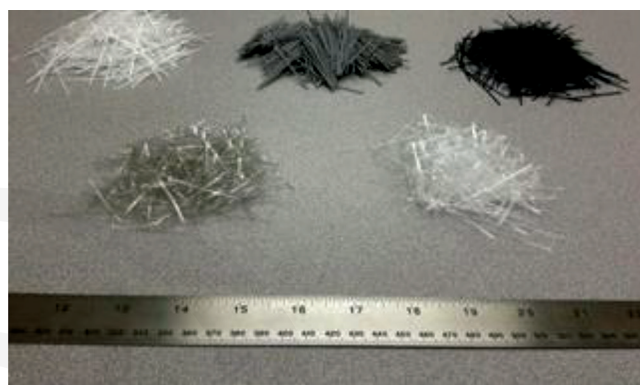
Fig. 2.1.7.4b—Fibers for use in shotcrete.
