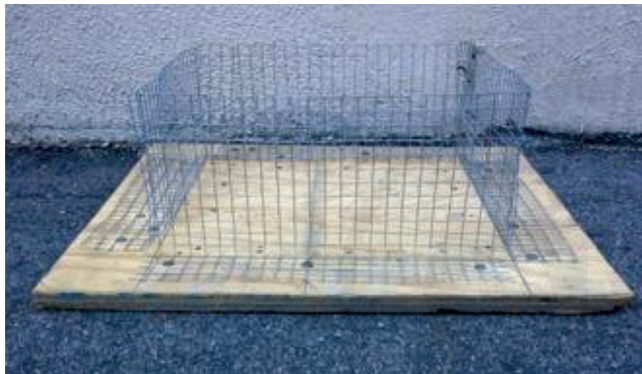
Fig. 1.6.3.1b—Material test panel with hardware cloth sides.
