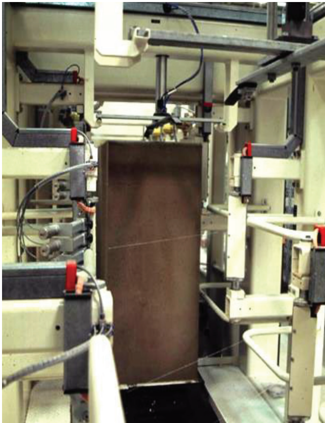
Fig. 3.4.3b—Cutting AAC into desired shapes.
