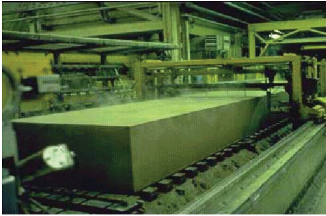
Fig. 3.4.3a—Fresh AAC after removal of molds.
