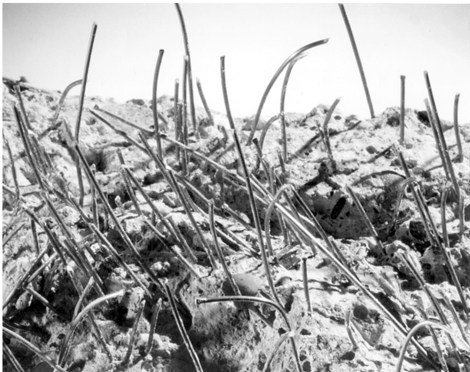
Fig. 2.1—Fracture surface of SFRC.
