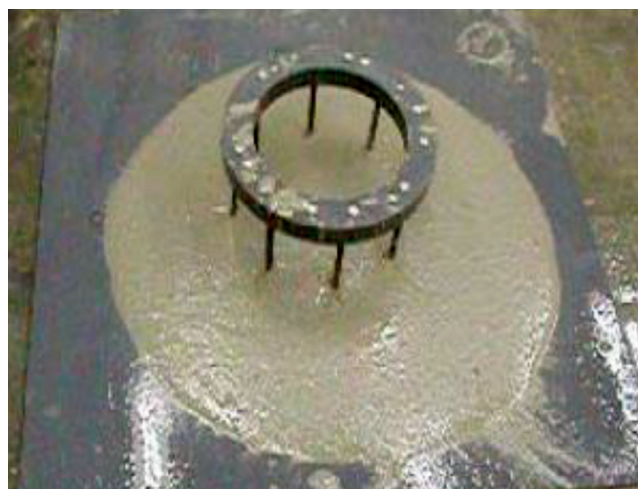
Fig. 3.2.2.4—Modified J-ring test steps employed by Kassimi (2013).
