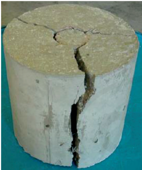
Fig. 5.3.3b—(a) Barcelona test failure mechanisms surfaces; and (b) specimen after testing (Molins et al. 2009).
