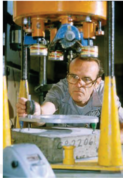
Fig. 3.6.5—Measuring depth of wear during ASTM C779 abrasion test. Note disks (Procedure A) and dressing wheels (Procedure B) at top of machine. (Courtesy of CTL Group.)
