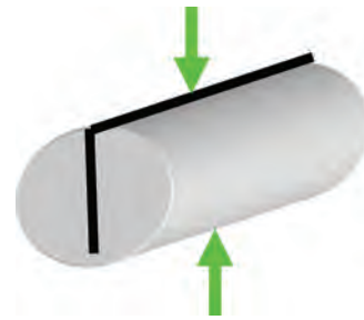
Fig. 3.3.7a—Schematic of splitting tension test setup (ASTM C307; C496). (Courtesy of BASF Construction Chemicals, LLC.)
