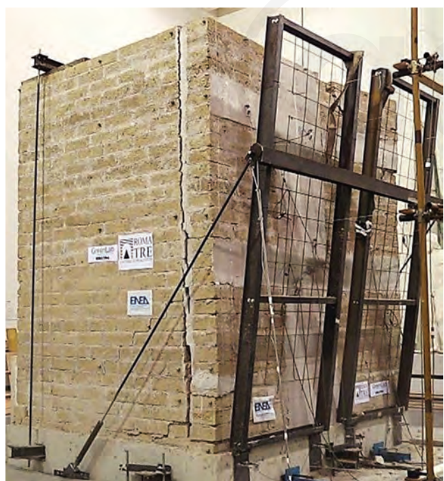
Fig. 3.4.1g—Shake table tests on masonry sub-assembly reinforced with SRG (De Santis et al. 2016a).
