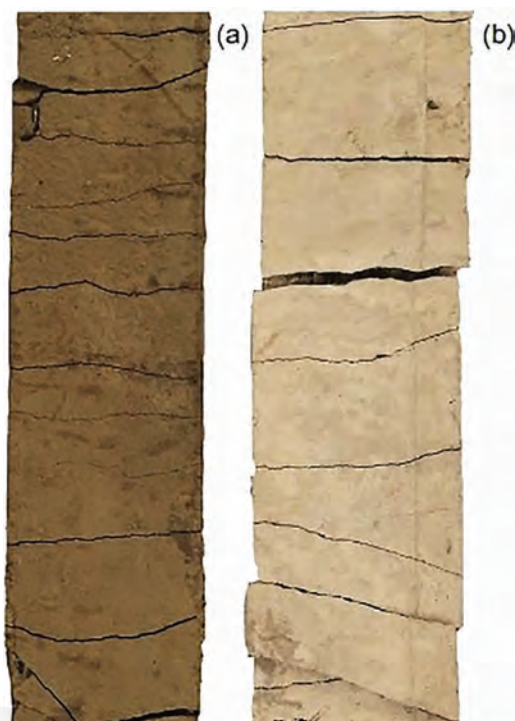
Fig. 3.3.1a—Crack pattern of SRG specimens with: (a) geopolymer-based matrixes; and (b) lime-based matrixes (De Santis and de Felice 2015b).
