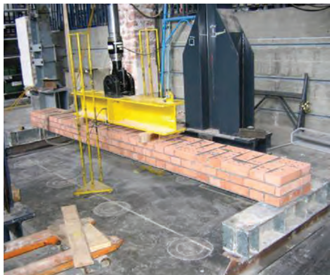
Fig. 3.4.1i—Experimental setup for four-point bending tests (Borri et al. 2009b).
