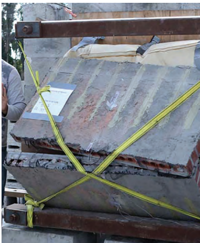
Fig. 3.4.1d—Crushing failure of the masonry panel reinforced with carbon FRCM/SRG (Babaeidarabad et al. 2014a).
