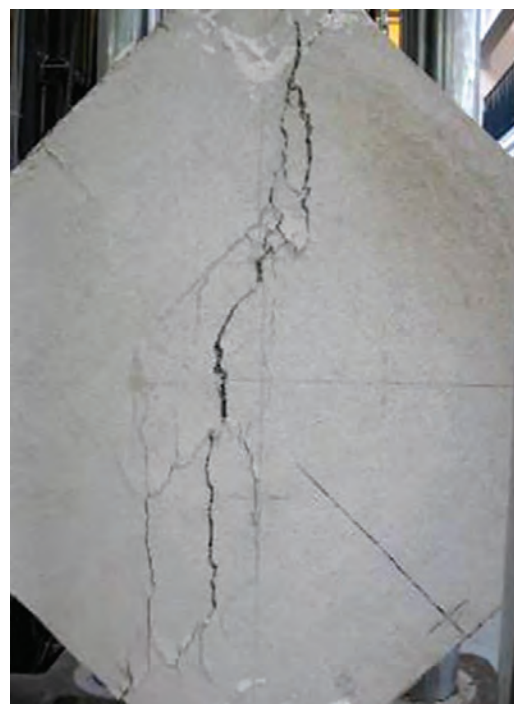
Fig. 3.4.2a—Shear failure by diagonal cracking of a tuff masonry panel reinforced with a basalt FRCM/SRG (Parisi et al. 2013).
