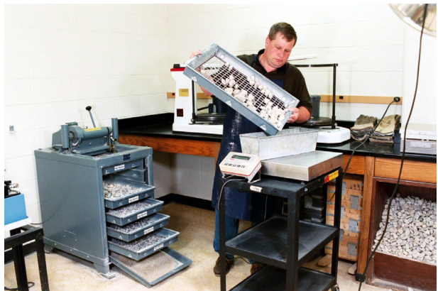
Fig. 2.5—Technician grading coarse aggregate (photo courtesy of PCA)
