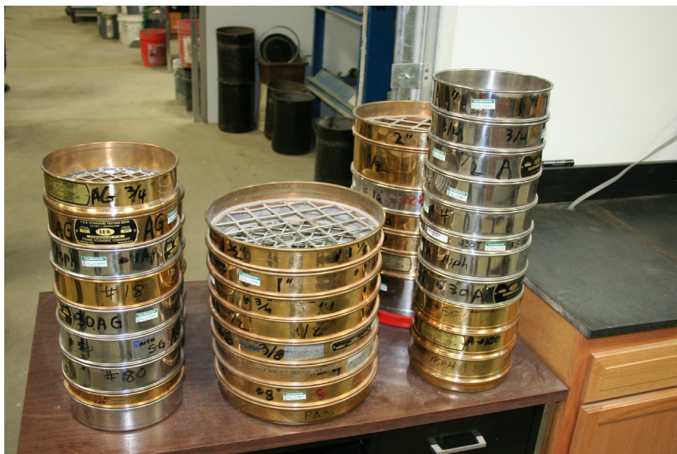
Fig. 2.6—Sieves are available in different size diameters; larger sieves (Fig. 2.5) are available for larger quantities of aggregate. Many sieves are available for use in a mechanical shaker
