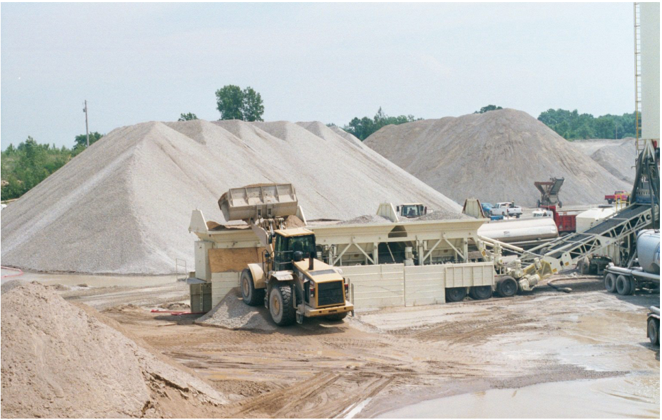
Fig. 2.8—Aggregate stockpiles should be kept clean and separate. Handling to minimize segregation is important (photo courtesy of PCA)
