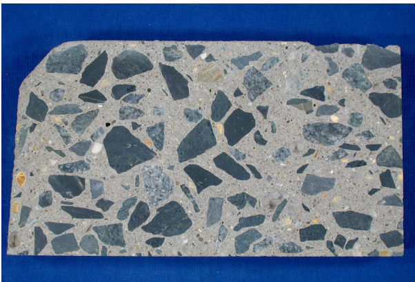
Fig. 1.3—Polished section sawed from hardened concrete. The cement-and-water paste coats each piece of aggregate and fills all spaces between the aggregate particles (photo courtesy CTLGroup)
