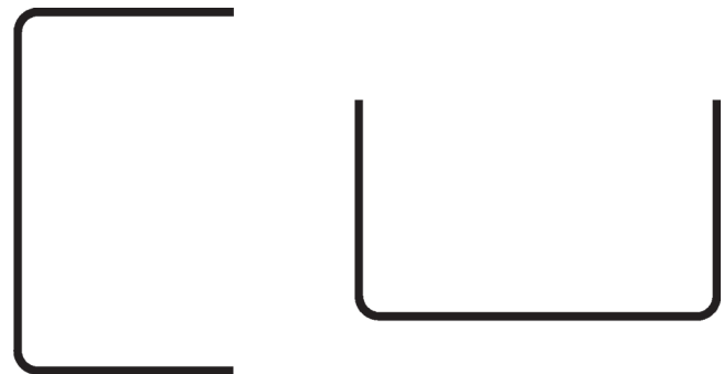
Fig. R2.3b—U-shaped transverse reinforcement.
