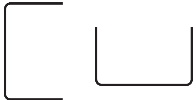
Fig. R2.3b—U-shaped transverse reinforcement.
