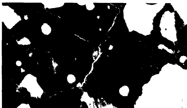
Fig. 2 — Fine fissures in the hydrated cement paste of the B-405 concrete.
