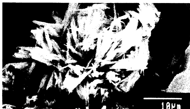
Fig. 11 — AFt needles in a vacant space.
