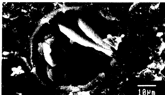
Fig. 5 — Hexagonal AFm plates in a large pore.
