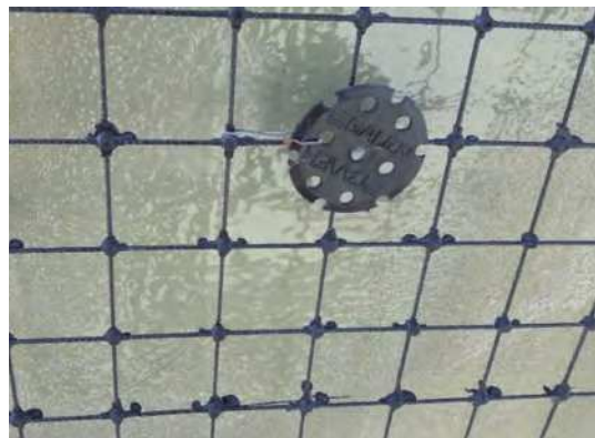
Fig. 2.2c—FRP grids used similarly to welded wire fabric for reinforcement of concrete slabs, walls, and other elements (photos courtesy Galen-Panamerica/Binevi)
