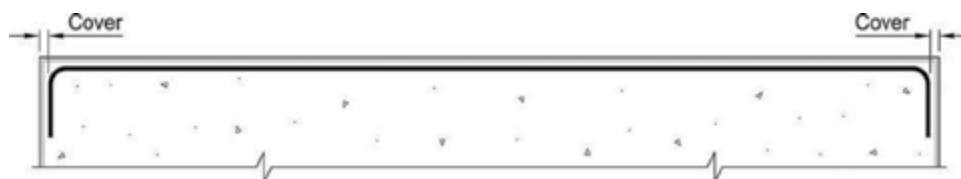
Fig. 3.2.7a—Single bar with hook at both ends.
