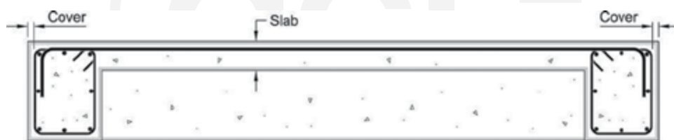
Fig. 3.2.7c—Substitution of two hooked bars with lap splice (lap splice shown offset for clarity only).
