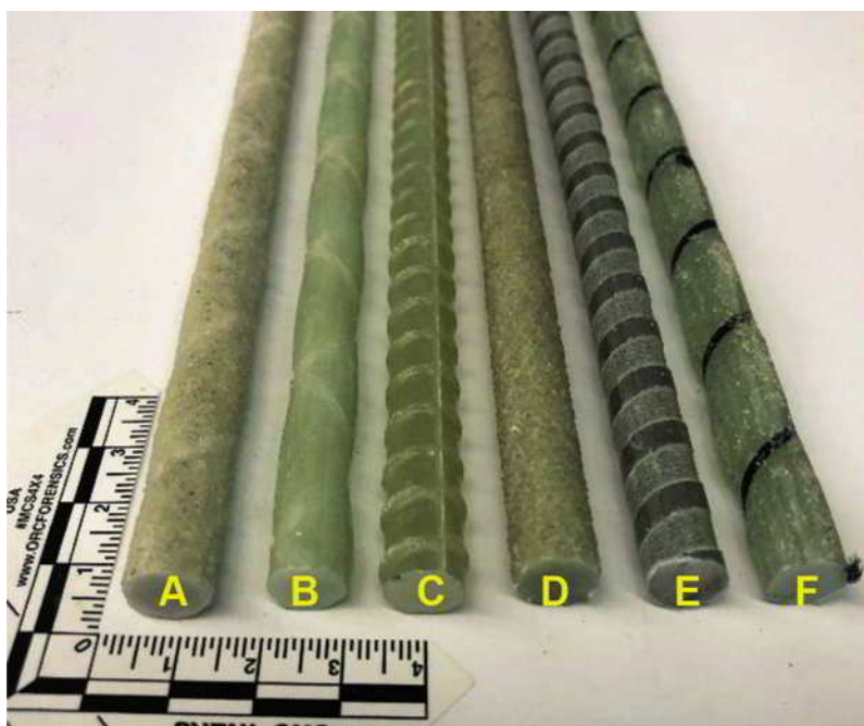
Fig. 4.1—Photo of different GFRP bars with various surface treatments including helically wound (b), sand-coated (d), sand-coated and helically wound [(a) and (f)], helically grooved or etched (e), and molded ribs (c).
